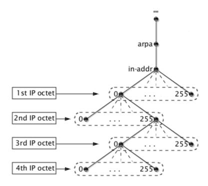
Therefore, to look up the FQDN associated with an IP address, the resolver simply has to query the name server for the PTR record (see <u>below</u>) of the corresponding node in the in-addr.arpa domain. For example, to get the domain name for the 62.149.140.23 IP address, the resolver will query the DNS server for the PTR record of the "23.140.149.62.in-addr.arpa" domain name.
