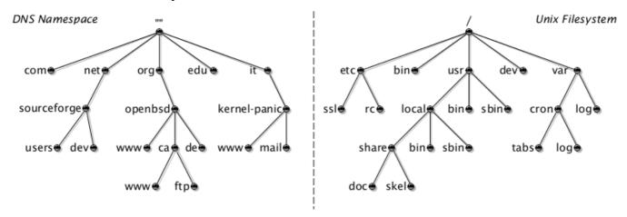
Each node in the Domain Name Space has a text label (the root node has a special zero-length label, "") and is uniquely identified by its domain name, i.e. the list of the labels on the path from the node to the root, separated by dots (Unix paths, on the contrary start from the root and are separated by slashes).
